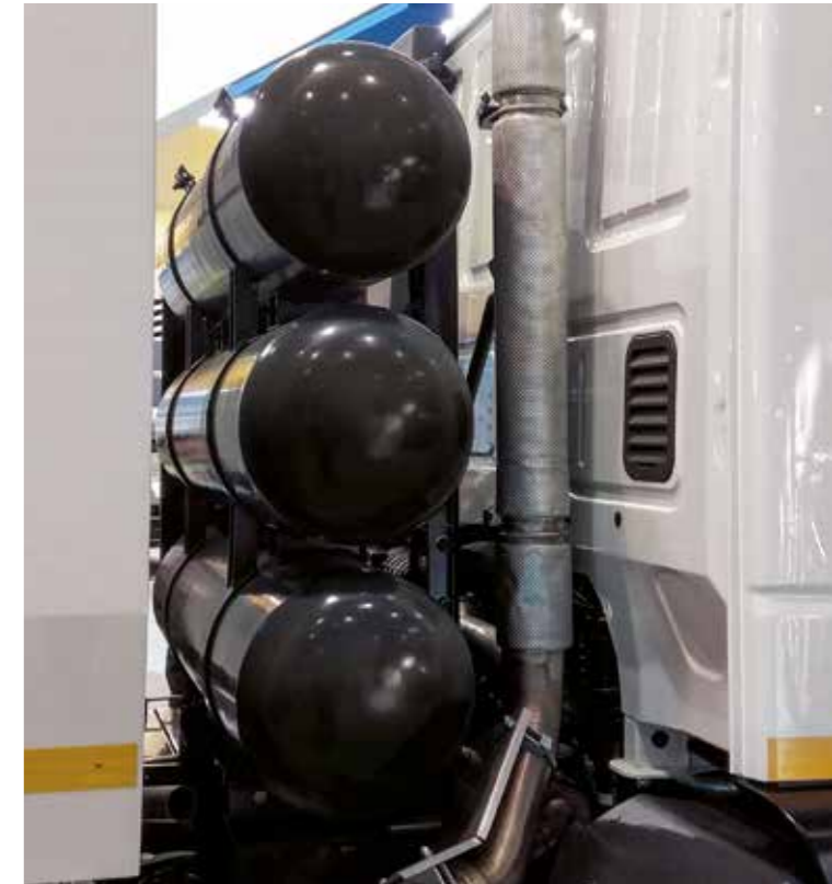
Rack behind the cab 420 litres / Up to 300km
